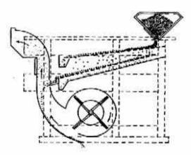
4. The grain passing over the bottom screen now enters the vertical air column of the blast fan where husks, chaff and light weight seeds are blown out while the full weight kernels pass down through the air blast and are delivered at the bottom of the cleaner as large, choice, full-weight grain.
