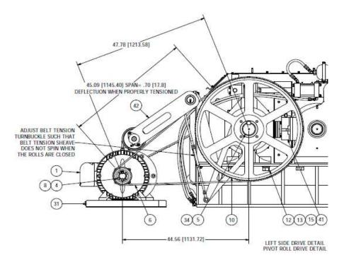
8. Make sure the motor guard back-plate is in place. Place the motor sheave and sheave taper lock bushing on the shaft. Tighten the bushing screws evenly until reaching the specified torque for the taper lock screws. See Table 1 on page 25 for correct torque requirements.
