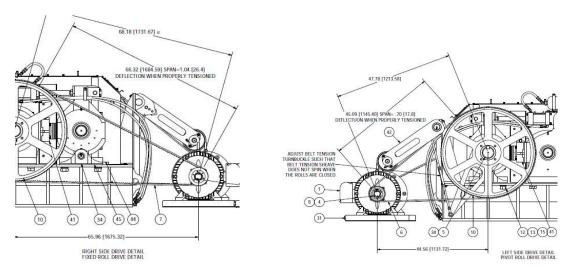
Step 4: Using a spring scale, apply a perpendicular force to any ONE of the belts at the midpoint of the span as shown in figure 2. Compare this deflection force with the values found in Step 3.
