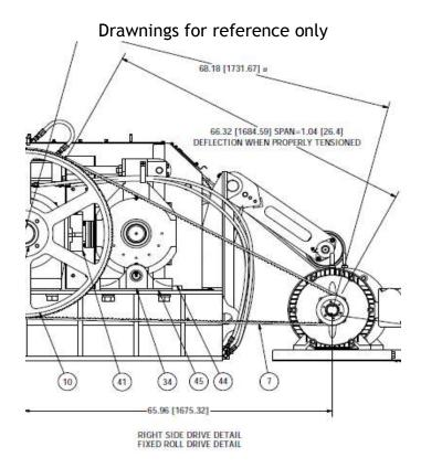
7. Place the motor over the bolts on the motor base or rails and install the washers and nuts. Do no tighten the motor bolts completely down.
