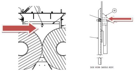
The roll end blocks or saddles are "V" shaped blocks made from aluminum or UHMW polyethylene. These are relatively soft materials and prevent damage to the roll ends should contact take place.
