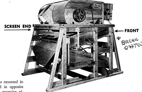
The Super 228-D has two 54" x 60" screens mounted in separate counter balanced shoes and pitched in opposite directions. This counter balancing eliminates excessive vibration and the screen arrangement enables the commodity to travel over the entire width and length of the screens giving better separation at high capacities. Each screen is individually adjusted in pitch.
